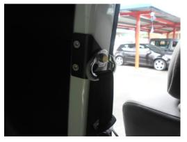
As the van you want to convert will be on an N1 Chassis, the aperture and reinforcing at the top of the C Pillar will not be present. Therefore we fit the BEBB Tested C Pillar Plate to the van to safely Carry the VW Seat Belt. We give you a certificate for the plate with every installation
